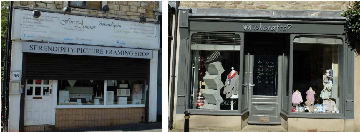
Figure 1: (Left) poor shopfront design. (Right) Attractive, well-proportioned traditional shopfront constructed from high quality materials with appropriate use of colours and restrained signage.
