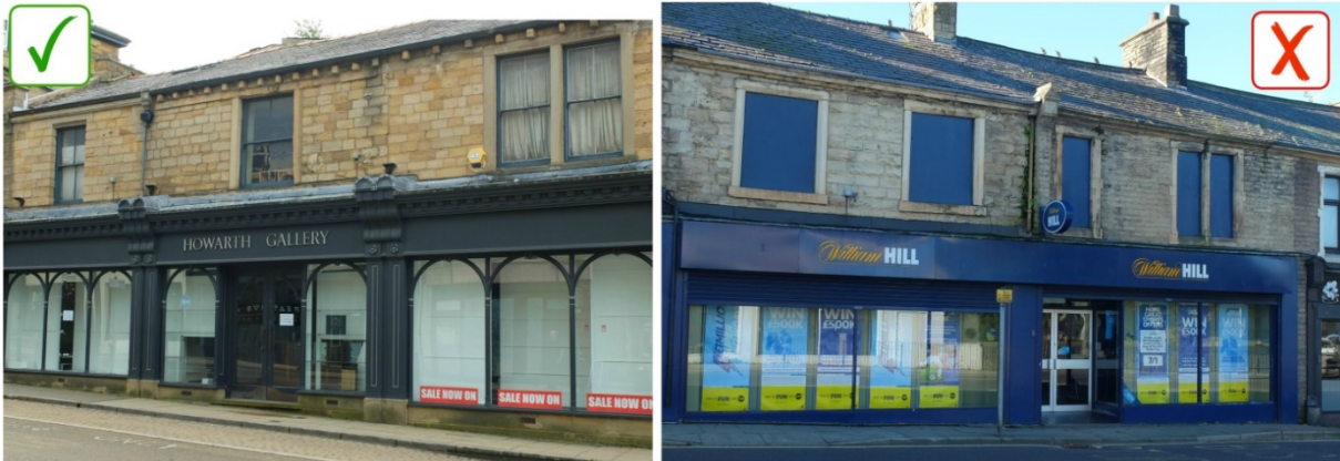
Figure 11: (Left) This shop extends across three units, but the fascia sign is appropriately broken into sections rather than extending across the whole shopfront. (Right) A continuous shopfront which extends across more than one property with wide horizontal format shop windows and disrupts the sense of verticality along the street. The blocking up of first floor windows further detracts from the visual qualities of the host building and the traditional terrace.
