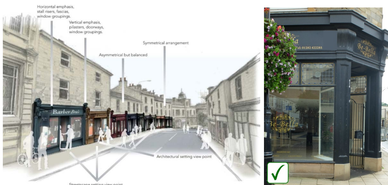
Figure 10: (Left) Example of a context assessment in Padiham Conservation Area. (Right) Corner shopfronts are visually important and can draw the attention of pedestrians on both streets.
